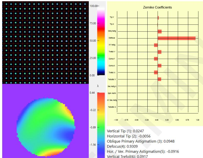
The WaveCamD is paired with DataRay's full featured software which has no license fees, unlimited installations, and free software updates. It's ideal for applications including: CW and pulsed wavefront measurements, zonal or modal wavefront reconstruction, field servicing of optical components and processes, one-shot beam alignment including pointing, beam collimation, and lens inspection.
