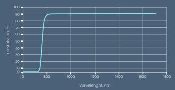
For optional use at higher than about 200 mW lasers (@1064nm) (does vary with wavelenght, refer to spectral sensitivity curve), you may consider using following filters to avoid sensor overfilling ("light flooding") issues and still ensure high visibility of your surroundings as the filter maintains high transmittance in the visible
