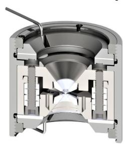
All SSDAC cells are Megabar-class DACs and with proper diamond culet size (<250  $\mu$ m), diamond alignment, and sample preparation the DAC can be routinely used in sub-Megabar and Megabar pressure range.
