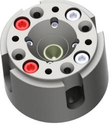
Boehler-Almax diamonds with 60° conical support and Tungsten Carbide seats.
