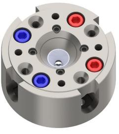
The DAC can be used with several diamond / seat combinations, but to make full use of the large symmetric opening the Boehler-Almax type diamond / seats with conical support are preferred. Because the diamond tilt in this DAC can be adjusted with a spherical seat base, the SSDAC is especially useful for cases where the diamond culets are not perfectly parallel to the bases of the diamond seats. The minimum 2x diamond + seat height for SSDAC-80 is ~10.5 mm.
