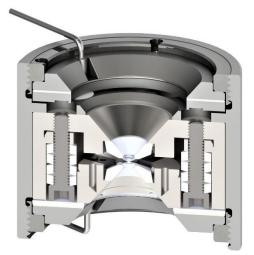
With proper diamond culet size (<250  $\mu$ m), diamond alignment, and sample preparation the DAC can be routinely used in sub-Megabar and Megabar pressure range.
