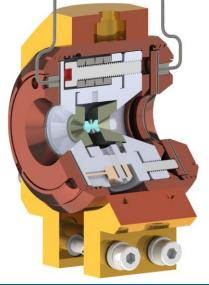
controlled by four M4 screws – either two left (LH) and two right (RH), or all RH screws on request. Nevertheless the DAC can be easily integrated with single or double membrane BeCu or Steel canister (compression and decompression) and fit into 47 mm (all versions) and down to 59 mm (shortened version) cryostat bores along and perpendicular the bore axis respectively.
