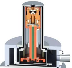
SD-type sensors (2 mm wide, 1 mm high): Two symmetric 2mm wide 1 mm deep cutouts go along the DAC body and two slots in the cylinder part normal to cylinder axis toward the piston. The sensor with Apiezon N grease can be inserted into the matching slot and secured with either G10/G11 (garolite) split ring or a nylon-tipped screws.
