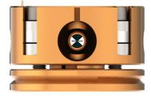
Another modification of the Standard Symmetric DAC is a Mini-Symmetric DAC with 40 mm Diameter. This DAC has smaller outside dimensions and is ~50% lighter than the full sized BeCu DAC. Nevertheless, the inner diameter and height of the diamond / seat area is the same and allows using "standard" sized diamond anvils and seats.
