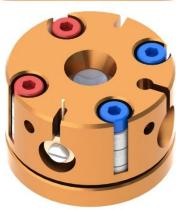
This DAC was designed for cryogenic work, with possibility of using it in strong magnetic fields, and therefore is made of non-magnetic BeCu alloy (C17200 / Alloy 25) with full-hard HT04 temper.
