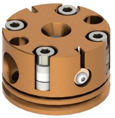
of the cell material and excellent thermal conductivity makes it optimal for use in cold-finger type cryostats, such as Physike Technology Scryo-S500 cryostat. Moreover, the design of the DAC allows to bolt the DAC piston directly to the cryostat cold finger, thus minimizing thermal losses, and conveniently attach temperature sensors, such as DT-670 in CU package, onto the DAC body close to the sample.
