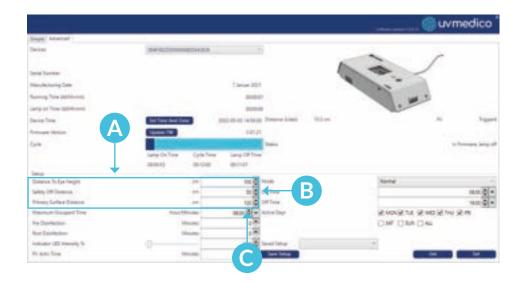
10) Save setup into template by pressing "Save Setup". D
