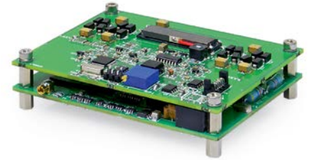
DQF-0.1-8 Pockels cell driver with integrated HV Power supply
