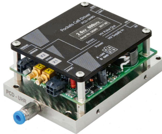
Figure 4. View of drivers DP-SP-250-3.6 , DP-SP-250-2.6 , DP-SP-500-2.6 , DP-SP-400-1.5 , DP-SP-1000-1.8 . Open PCB version.
