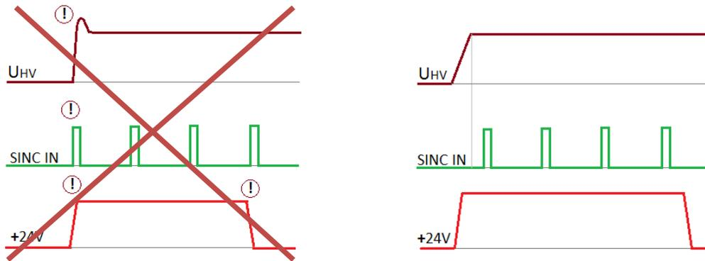
***Incorrect driver operation.*** SYNC IN pulses appears before HV and 24V; SYNC IN pulses continues after 24V is switched off; HV supply gives an overshoot.
