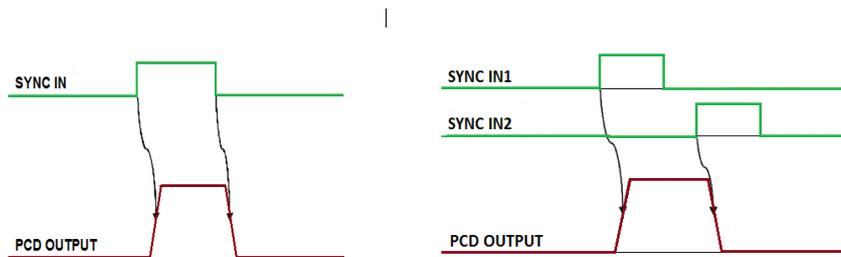
**Figure 5. Control timing principle charts with 1 sync pulse (Mode 1, left) and with 2 sync pulses control (Mode 2, right)**
