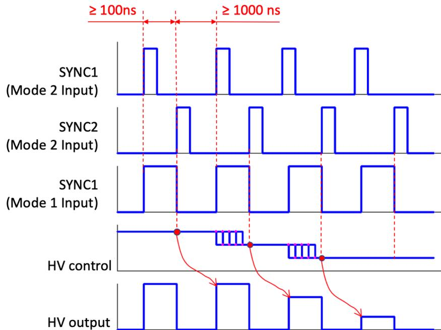
**Figure 7.** HV Control principle timing chart. Either Mode 1 or Mode 2 is used for control
