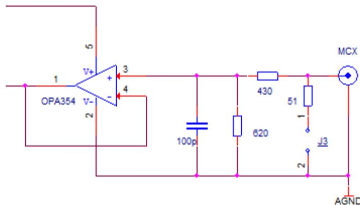
**Figure 6. HV Control input circuit**
