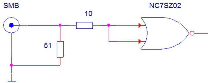
**Figure 4. SYNC input circuit**
