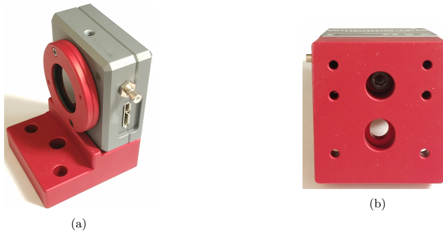
Figure 3: (a) The WinCamD-LCM is placed on the mounting block as shown. (b) A #8-32 screw fastens the WinCamD-LCM to the mounting block.
