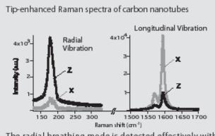
The radial breathing mode is detected effectively with z-polarization. ZPol provides a new detection technique sensitive to molecular orientation in 3D. Reference: Y. Saito et al., Chem. Phys. Lett. **410**, 136 (2005).
