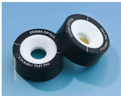
Potassium titanyle arsenate ( $\text{KTiOAsO}_4$ ), or KTA, is a nonlinear optical crystal for Optical Parametric Oscillation (OPO) application. It has good nonlinear optical and electro-optical properties, e.g. significantly reduced absorption in band range of 2.0 – 5.0  $\mu\text{m}$ , broad angular and temperature bandwidth, low dielectric constants.
