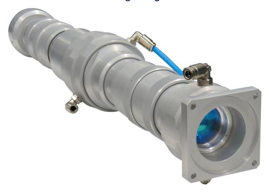
With these unique devices it is possible to convert a divergent  $TEM_{00}$  or multimode laser beam from a fiber laser into a collimated Flat-top beam with nearly 100% efficiency and conserving flatness of the wavefront.
