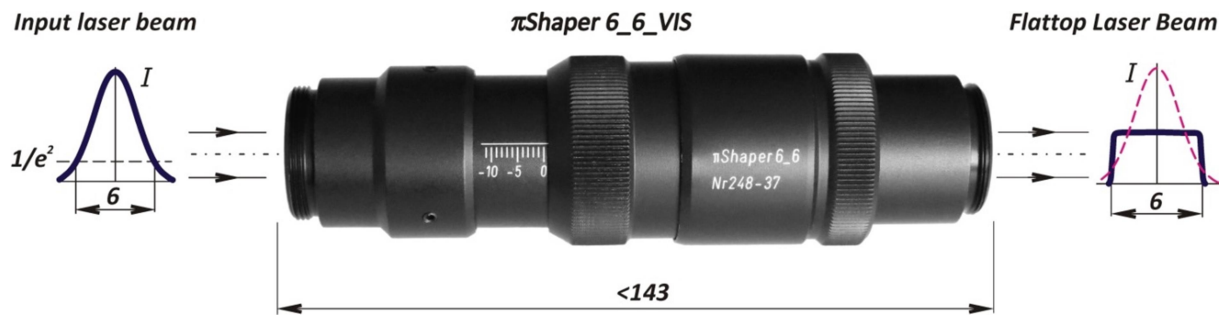
Figure 4. \pi Shaper operation.
