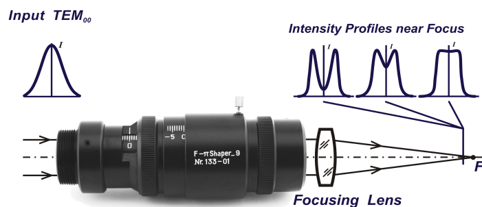
Fig. 2 Principle of the Focal- \pi Shaper operation.
