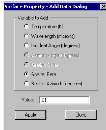
FIGURE 3.25 - Adding a new value of |\beta-\beta_0| to the BSDF table.
