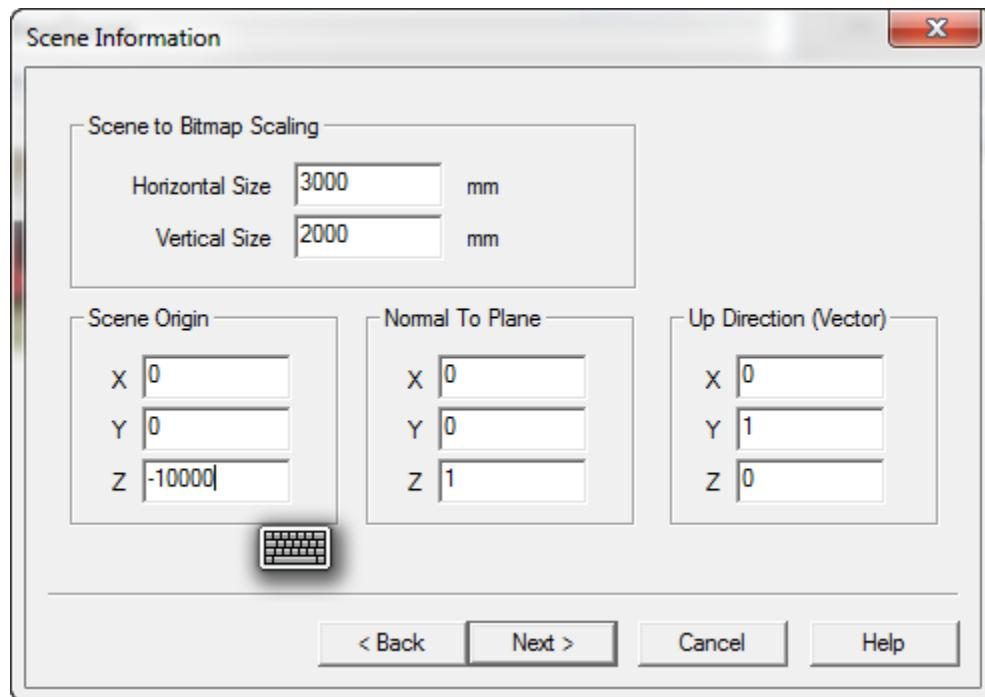
The lens in **lensdemo.oml** is near the origin of coordinates and has its optical axis along the z axis, so we put the origin of the scene 10m away (at  $z = -10,000\text{mm}$ ) and on the z axis ( $x = 0, y = 0$ ). We orient the scene so that it is perpendicular to the z axis (*Normal to Plane* = 0,0,1) and has the y axis pointing up in the scene (*Up Direction* = 0,1,0). Click *Next* to go to the next pane.
