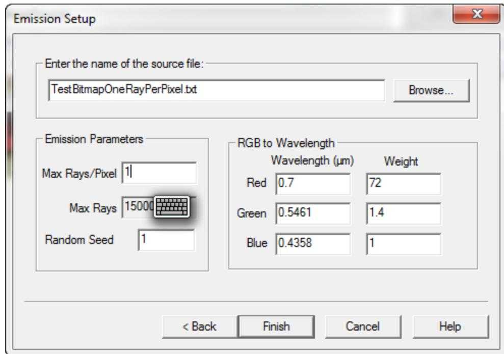
The actual number of rays generated depends on the Red, Green Blue value of each pixel. The Bitmap Source Module will adjust the number of rays for each pixel for each color so that the flux for each ray is approximately the same. Pixels that are black will generate no rays.
