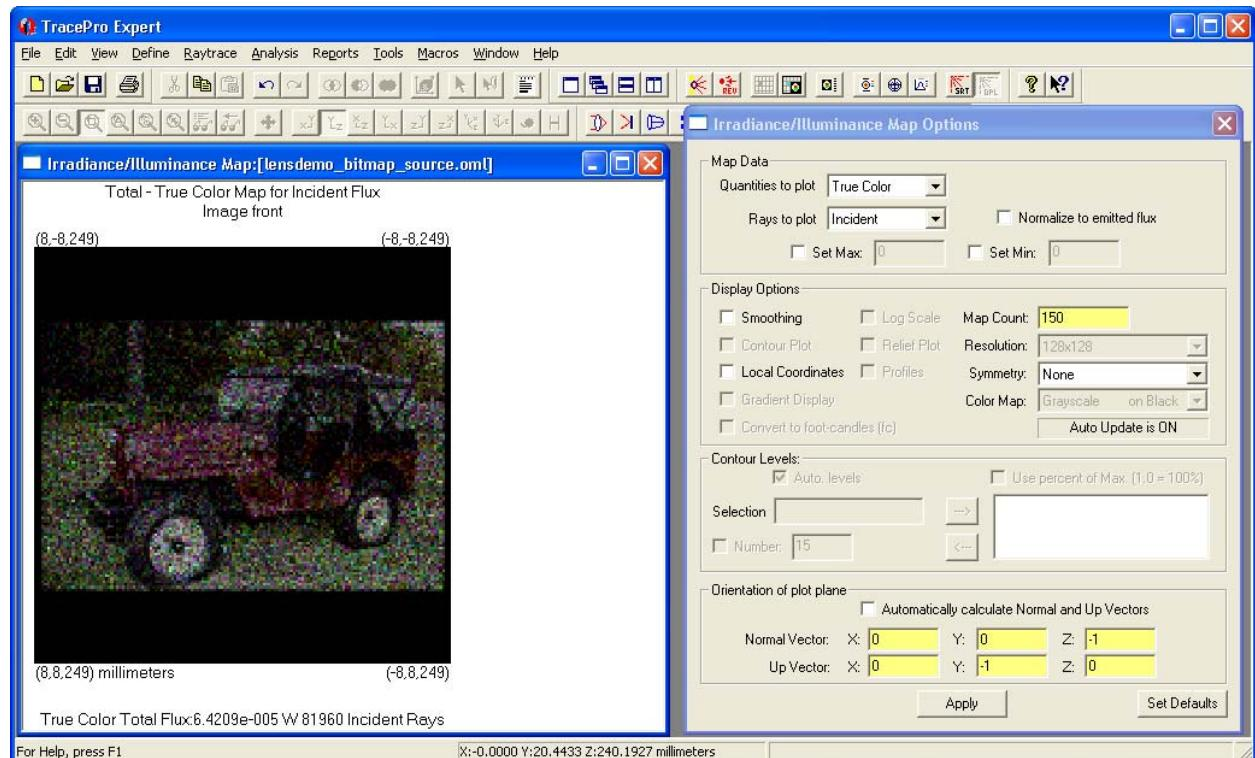
Clearly, many more rays are needed to obtain an image that has tolerable signal-to-noise ratio. We have repeated the exercise with ten times as many rays. The Bitmap Source module was run
