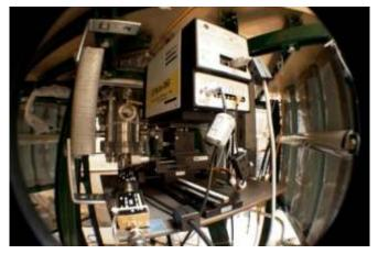
The 4 Picos ICCD camera integrated at the experimental setup of the dense plasma focus with the from the backside facing the window of the vacuum chamber. Figure reprinted with permission of the Lawrenceville Plasma Physics, Inc (2012).
