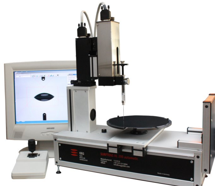
SURFTENS HL 200 with motorized dosing unit and motorized drop placement, both motorized movements are software controlled
