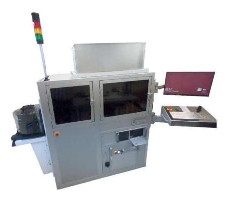
Fully automatic contact angle measuring instrument with 3 axis wafer handling robot, loadport for 300 mm FOUP and SECS/GEM interface
